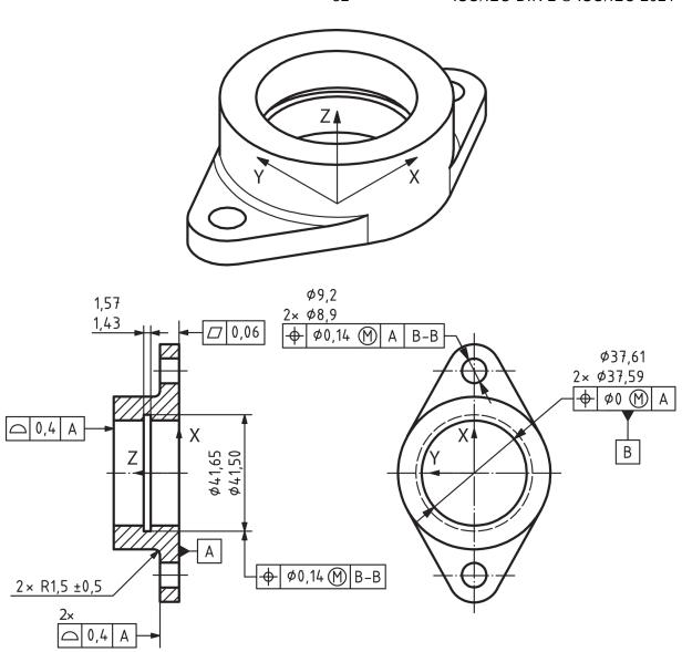
Figure 7 – Example of a mechanical engineering drawing
