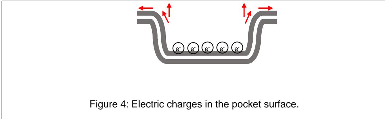
As shown in Figure 4, the path of charge dissipation that is most important is along the top-side surface of the planar material.
