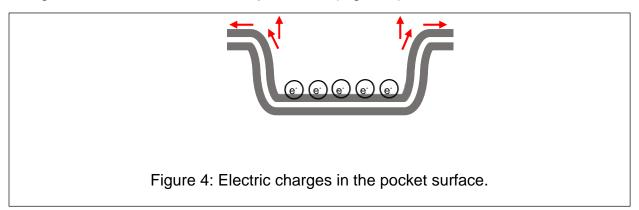
As shown in Figure 4, the path of charge dissipation that is most important is along the top-side surface of the planar material.
