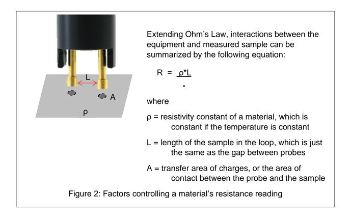
The above is based on surface resistance ( $\Omega$ ), but can easily be converted to surface resistivity ( $\Omega$ /sq). As defined in ANSI/ESD STM11.11 (Surface Resistance Measurement of Static Dissipative Planar Materials), to convert resistance from ohms to ohms per square (surface resistivity) multiply the reading results by 10 (or alternatively if reporting in scientific terms, increase by one full decade. Example: from 1.0x10^5  $\Omega$  to 1.0x10^6  $\Omega$ /sq). See Figure 3
