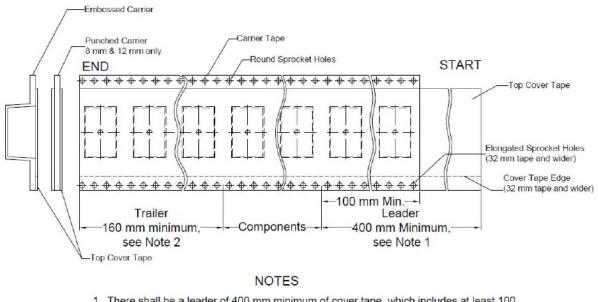
There shall be a leader of 400 mm minimum of cover tape, which includes at least 100 mm of carrier tape with empty compartments and sealed by the cover tape. All of the leader may consist of the carrier tape with empty compartments sealed by cover tape.
